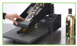
With the built-in LED display users can easily set-up variable spacings, save up to nine different container offsets and see the number of applied labels.
